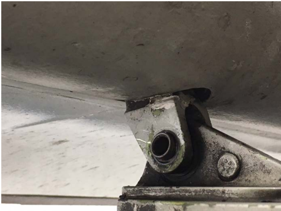
Pic 2: Bushing remains in fitting holding flap in place
