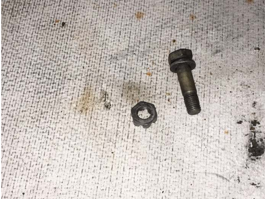
Pic 1: Bolt and nut found in flap canoe
