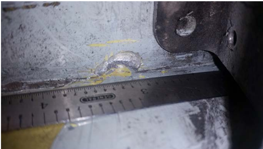
Figure 2 – Damaged area during blend-out
