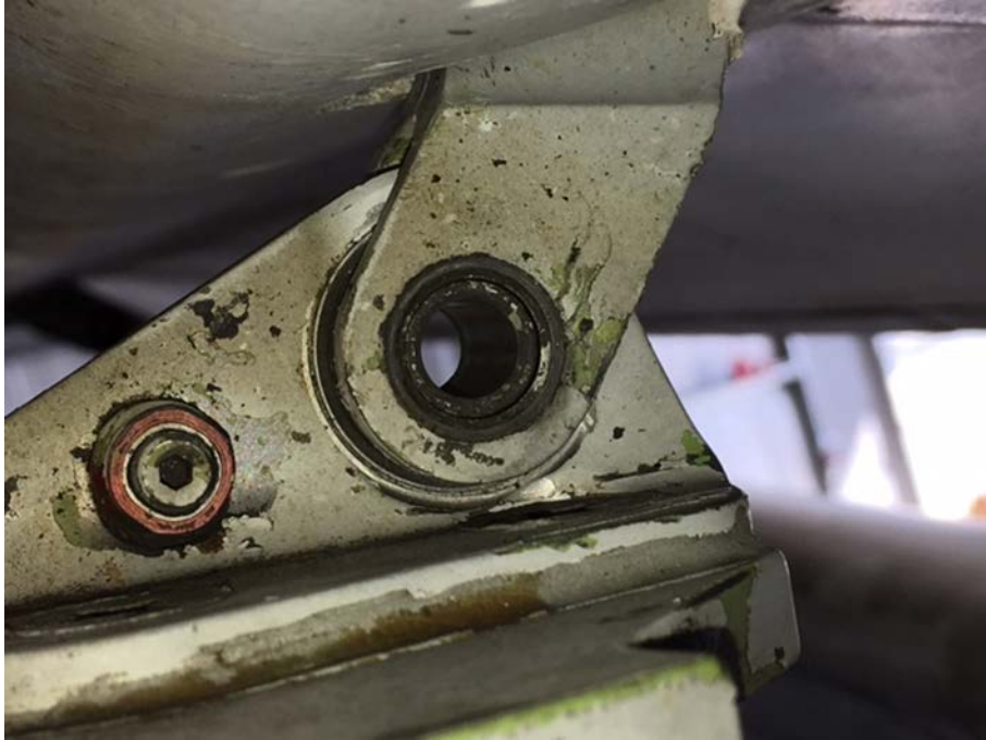
Pic 3: Bushing in fitting
