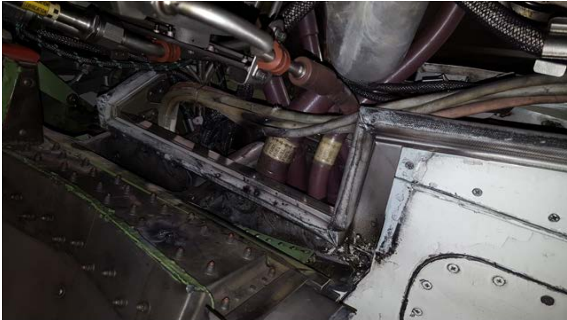
Fig 1: RJ900 - Nacelle location of wire chafing on panel fasteners
