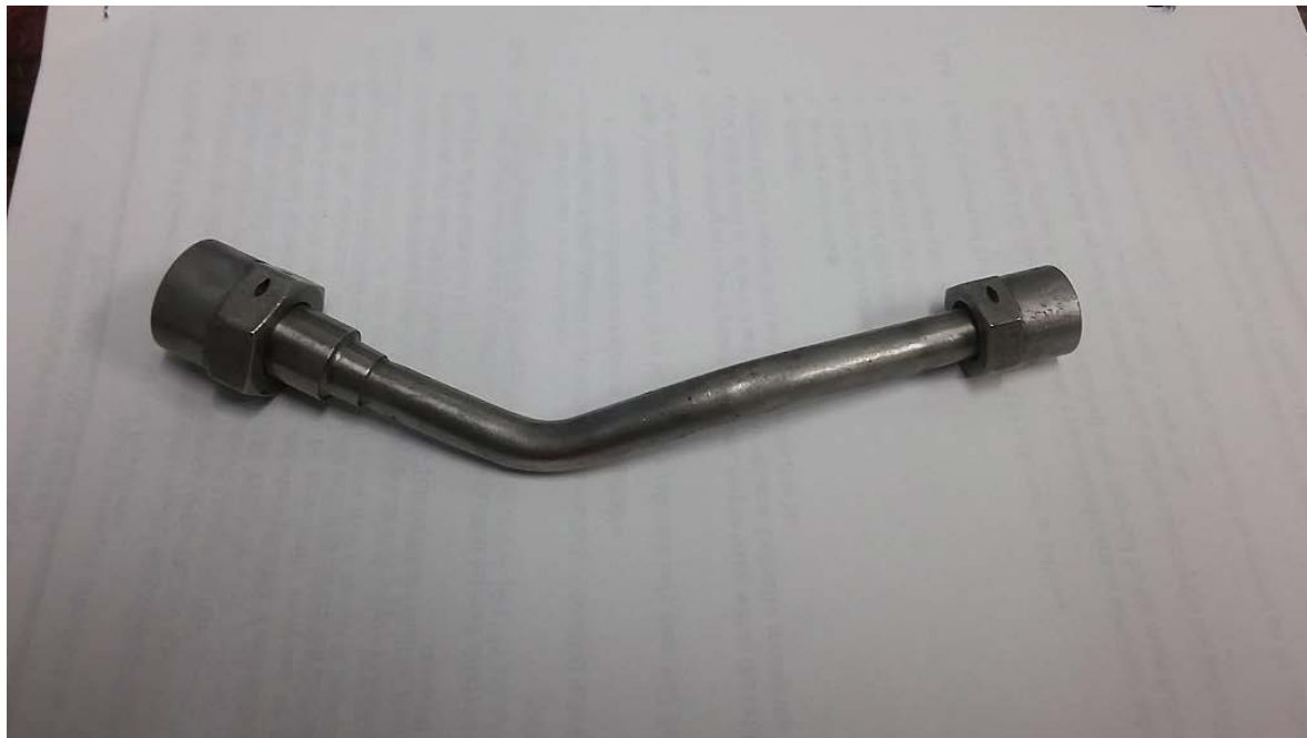
Cracked Fuel line
