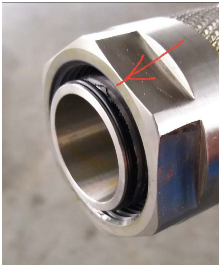
Fig 2: O-ring shown installed in suction line from previously removed engine
