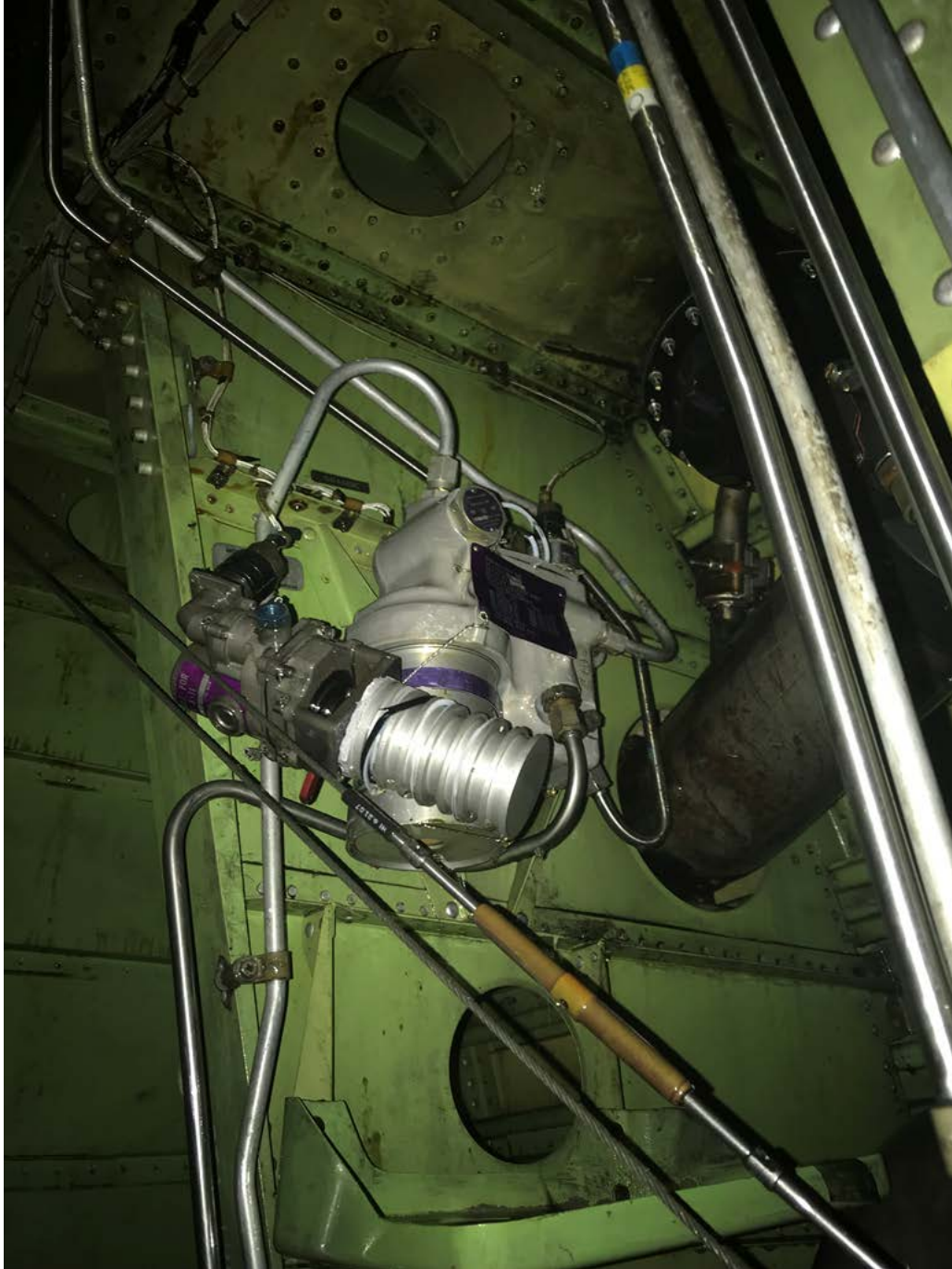
Picture 2: Valve found hanging beside module assembly
