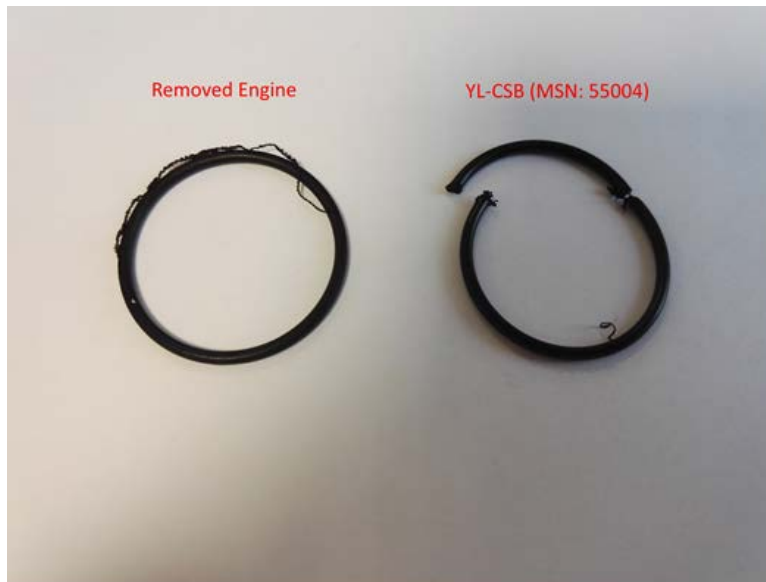
Fig 1: O-ring from subject aircraft and o-ring from another engine previously removed
