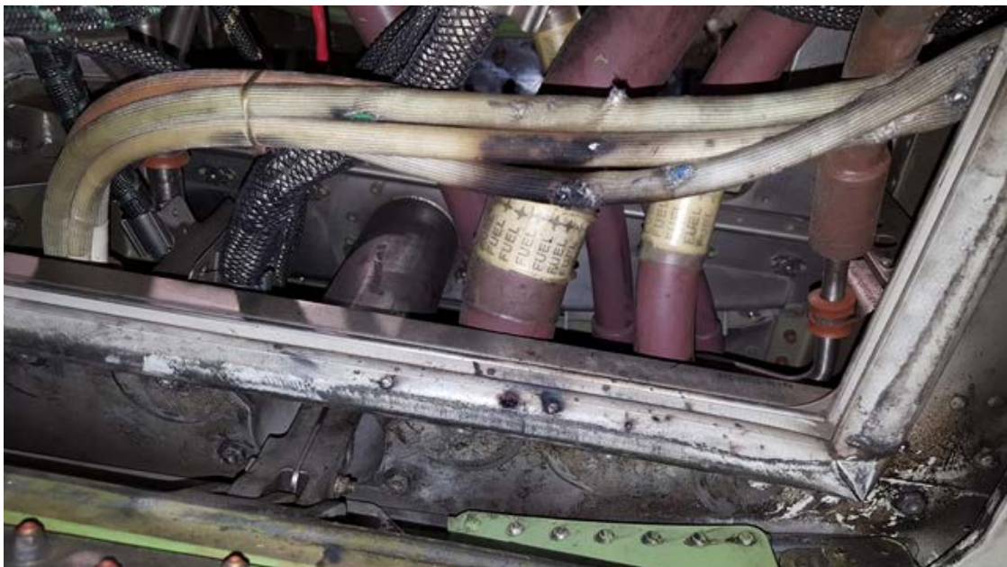
Fig 2: RJ900 - Burnt wires next to fuel line
